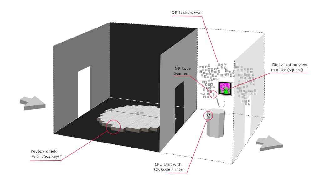
\* Keyboard field consists of 89 mechanical keyboards, which are mounted on aluminium chassis. To facilitate transportation only keyboards needs to be transported, while the aluminum structure can be constructed in-situ. Same applies to CPU booth.
